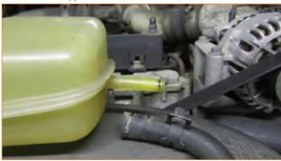
7. Remove the lower coolant overflow reservoir hose and the lower radiator hose. Pull the coolant overflow reservoir up and out of the vehicle.
