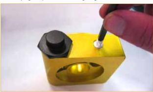
**4.** Wrench tighten the plug 2-3 full turns. (1/8"npt only)
