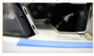
**4.** Reinstall the two hidden pop clips on the bottom of the front bumper, then reinstall the side splash shields and secure them to the bumper using six pop clips.
