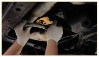
**2.** Attach and route the upper oil cooler line. Feed this line up between the exhaust manifold and the frame of the car, and then feed the other side of the line between the body and the headlight.
