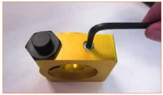
5. Remove any excess Teflon® after tightening.
