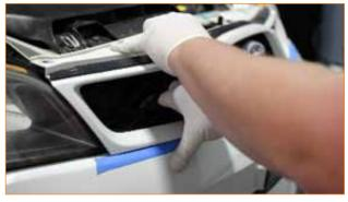
**6.** Remove the two hidden pop clips from the bumper. The clips are behind the side grille inserts.
