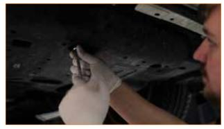
8. Check the oil level and refill the oil as needed.
