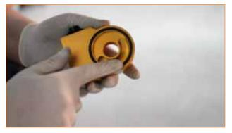
3. Attach the sandwich plate adapter to the oil filter housing.
