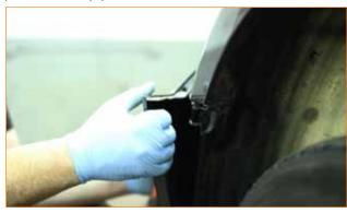
**6.** Unbolt the horns and attach the horn relocation bracket. The relocated horns should both be on the driver's side of the vehicle.
