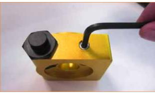
5. Remove any excess Teflon® after tightening.
