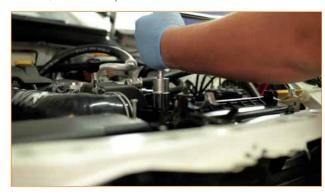
${f 10.}$  Install the oil lines onto the sandwich plate. Tighten down all the oil line fittings.
