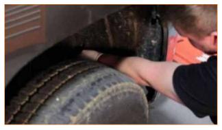
**2.** Locate the lower radiator hose on the base of the passenger side of the radiator. Loosen the clamp and slowly slide the hose off the radiator. This radiator does not come from the factory with a drain plug, so the fluid must be drained from the lower hose. Allow all fluid to drain from the radiator.
