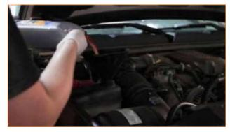
7. Start the vehicle and set the heat to high to purge the cooling system of any air bubbles. Allow the vehicle to reach operating temperature and check for any leaks.
