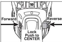
For **reverse** (counterclockwise) rotation, push in the control switch from the left side of the tool. **Check direction of rotation before use.**
