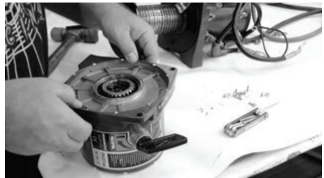
1-5: Place Gear Housing Leg in the angle desired, and screw in bolts.
