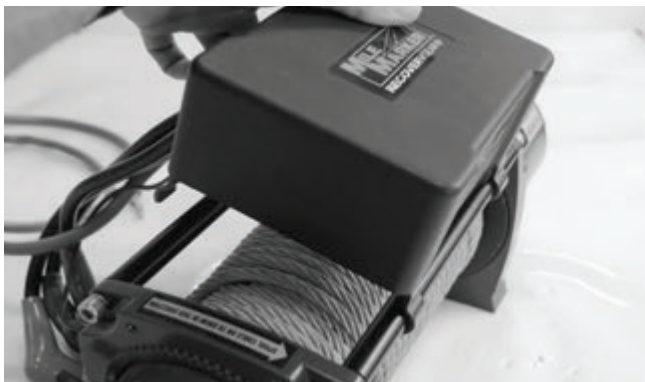
2-9: Mount Control Box on the Tie Bars.
