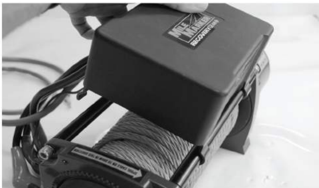
2-9: Mount Control Box on the Tie Bars.
