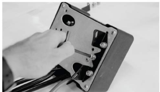
2-2: Install the mounting bracket to the bottom of the control box with a 10mm wrench.
