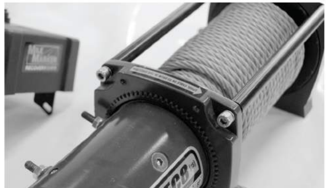
2-4: These are the mounting points where the bracket will be screwed in.
