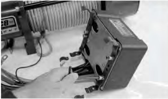
2-8: Install the mounting bracket to the bottom of the control box with a 10mm wrench.
