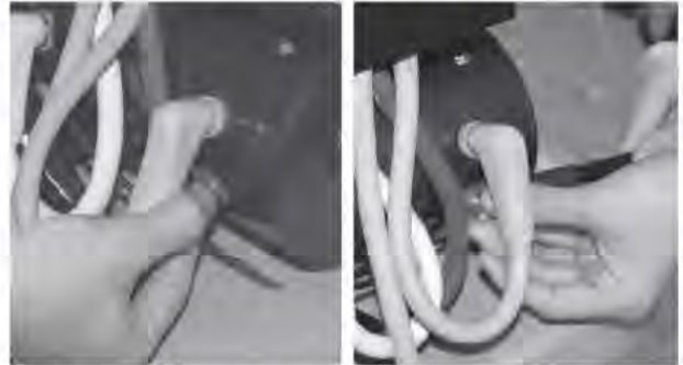
2-13: Black Cables (ground): Remove bolt, Attach both large and small cables, and return bolt to motor.
