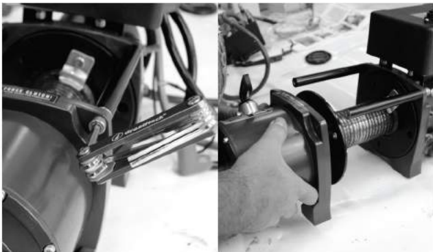
1-2: Unscrew and remove Gear Housing from Tie Bars.
