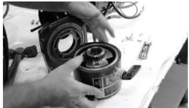
1-4: Separate Leg and Gear Housing.
