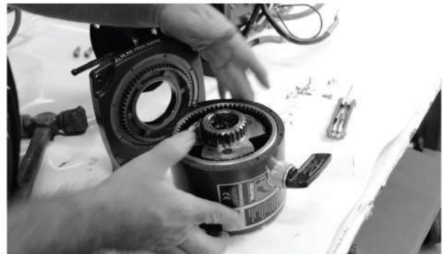
1-4: Separate Leg and Gear Housing.
