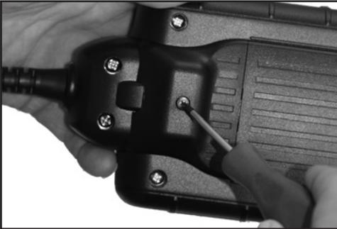
3. Grasp the housing and firmly pull the cable assembly from housing.
