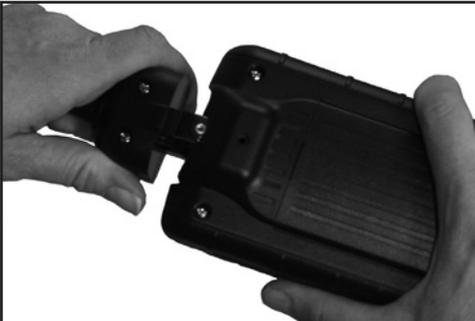
4. To attach a new cable, align the cable and tester housings and push together. Insert the screw and tighten.
