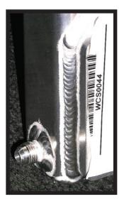
This photo shows a port welded into the lower tank of the radiator, just before the water pump, as a low pressure return connection.
