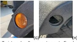
9. Twist and pull connector out. Feed connector and leads between outer and inner fender panels into mount hole. Slide light up into location and snap retaining clip in. This will take force. Reinsert connector back into side light housing and twist to lock in. (I)
