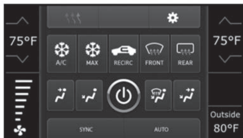
Automatic climate controls
