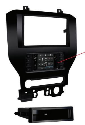
Built in interface in the touchscreen display allows either the factory camera or aftermarket camera through the touchscreen display.
