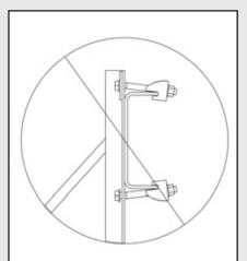
WARNING DO NOT MISALIGN BOLTS BOLTS MUST BE PARALLEL TO THE FRAME RAIL FLANGE
