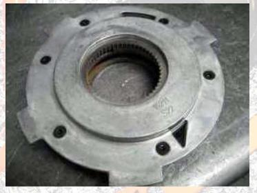
19 Here is the stock pump assembly removed from the transfer case for the upgrade installation.
