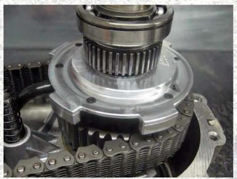
25 Begin to reassemble the transfer case by reinstalling the pump, reluctor wheel and support bearing on the main shaft followed by the snap ring. (Verify that the stepped edge of the reluctor wheel is facing the pump and that the snap ring groove in the bearing race is on the top side of the bearing as shown.) Then reinstall the pickup tube in the pump housing making sure that the O-ring is intact and properly positioned.
