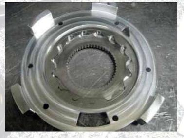
23 Use the supplied blue threadlocker to apply a small drop on the threads of each of the six screws that hold the pump together as shown.
