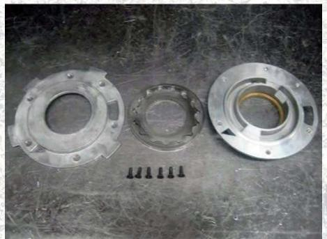
21 Using a T-15 Torx screwdriver or bit remove the six screws holding the pump together. This image shows a disassembled view of the pump. Clean and dry all parts. The pump body may be discarded, (top plate of the pump only, the gear set, screws and bottom will be reused), as it will not be reused.
