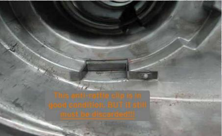
15 Hopefully this is the condition of your anti-rattle clip and no damage has been done to the rear case half. The one shown here was in excellent shape and shows no abnormal signs of wear. NOTE: The anti-rattle clip must be removed and discarded regardless of its condition as it is no longer necessary and cannot be used with the Merchant Automotive Transfer Case Pump Upgrade kit!
