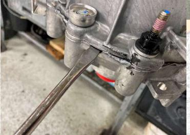
13 Gently pry the case halves apart with a large flat blade screwdriver or similar pry tool in the recessed notches on each side of the transfer case as shown.
