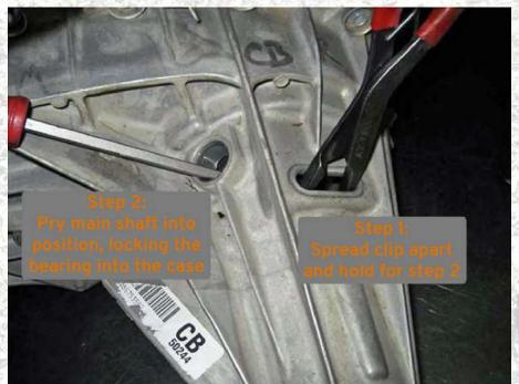
31 Spread open the snap ring through the access hole in the rear case half while using a large flat head screwdriver or similar pry tool to slide the mainshaft support bearing into place locking it into the rear case housing.
