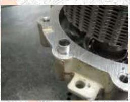
27 Locate the dowel pins (they could be in either half of the transfer case housings) and place them in the front half of the transfer case. One dowel pin is required on each end of the transfer case; the location is identified by the counter bore in the case half. BOTH of the dowel pins MUST be installed or severe damage to the transfer case could occur.
