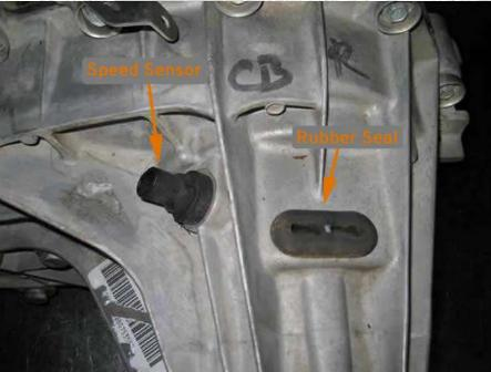
Of Viewed from the top of the transfer case you will find the output speed sensor as well as a rubber plug.
