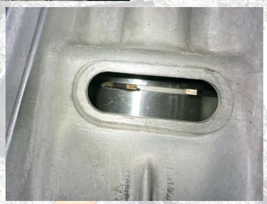
23 Reinstall the speed sensor and rubber plug. A small amount of the silicone sealant can be applied to the threads on the sensor as well as around the rubber seal for a tight leak proof seal. To complete the upgrade, reinstall the transfer case drain and fill plugs. For additional protection we recommend using the Merchant Automotive Transfer Case
