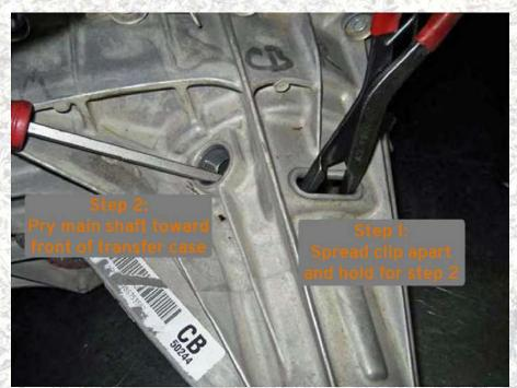
11 Using snap ring pliers and a large flat blade screwdriver or pry tool, open the snap ring then gently pry on the reluctor wheel pushing it forward toward the front of the transfer case. This will release the rear support bearing from the rear case housing.
