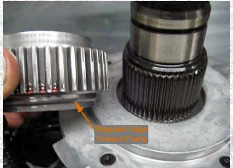
17 After the bearing is removed slide the reluctor wheel up and off the main shaft. Notice the orientation of the wheel, there is a stepped edge on the lower side of the wheel that MUST be reinstalled toward the pump.
