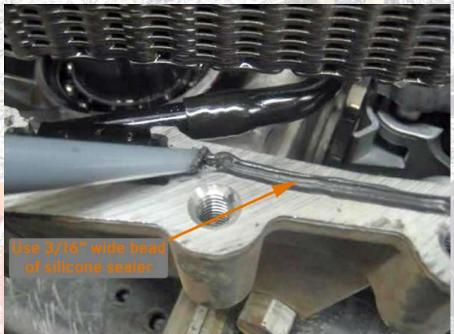
29 Use the supplied silicone sealer with the applicator nozzle and apply a 3/16-inch wide bead of silicone sealer around the perimeter of the case in the center of the sealing surface flange. It is not necessary to go around the bolt holes; apply the sealer to the inboard side of the bolt holes as shown.
