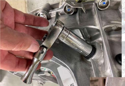
O9 Next use a 19mm or 3/4-inch box-end wrench or deep socket to remove the speed sensor. DO NOT use an impact gun, on the speed sensor, it is plastic and will break.
