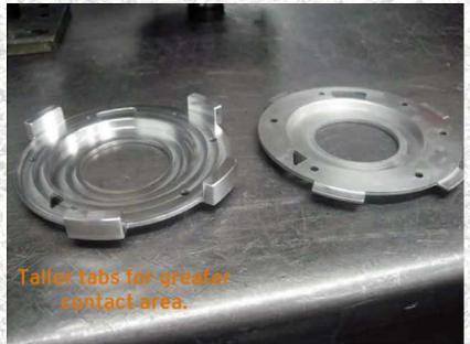
O1 The differences are quite obvious between the upgraded Merchant Automotive pump body over the stock unit. The MA part is CNC-machined from aircraft quality T-6061 aluminum with precision tolerances of less than 0.0001-inch. The larger tabs provide more surface area on the case to virtually eliminate rub through.
