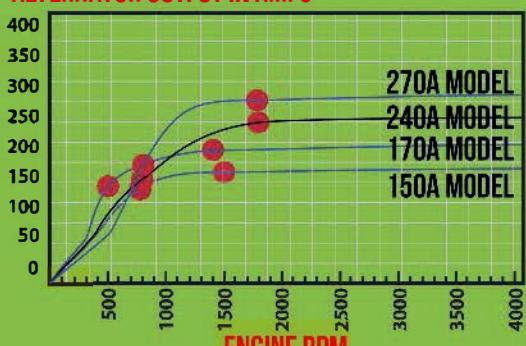
\* ENGINE RPM SPECS ASSUME A 7" DIAMETER CRANK PULLEY
