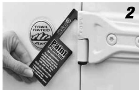
**2** On the upper door hinge, hang/place paint protector centered just below the hinge nut. For some YJ models use painters tape to hold in place.
