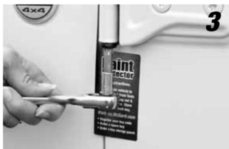
**3** Using the appropriate driver, socket, or bit, remove the hinge nut.
