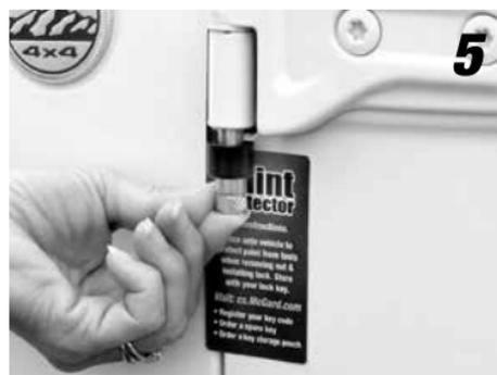
**5** Thread the lock into hinge by hand.
