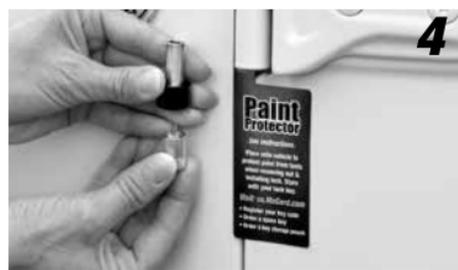
**4** Insert key tool into hinge lock and engage lock nut pattern.
