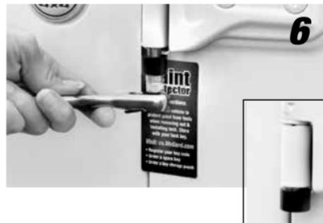
**6** Using a 1/4" ratchet and key tool, tighten the lock to approximately 80-90in.lbs. Do not over-tighten. Remove key tool and paint protector. Repeat process on other doors (one lock per door).
