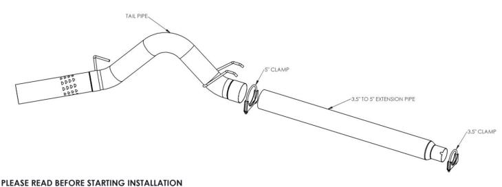
MBRP Inc. has made every effort to ensure that all components of this system are of superior quality and properly packaged. It is the installer's responsibility to ensure that all components are present and tit together as shown. Please also ensure that all components are undamaged before removal of the factory exhaust. Finally, check that this system properly matches the make and model of the vehicle and will not interfere with previous or planned modifications.
