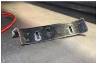
4) PUSH YOUR NEW MAX TRAC CROSS MEMBER UP TIGHTLY AGAINST THE ORIGINAL CROSS MEMBER AND CLAMP IT. ALSO INSTALL THE BOLTS ON THE VERTICAL SIDE OF THE CROSS MEMBER TO HELP HOLD IT IN PLACE.
