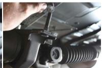
2) HOOK A TAPE MEASURE ON THE ORIGINAL CARRIER BEARING SLOTTED HOLE AND DRAW A LINE 3"OUTWARD: REPEAT ON OTHER SIDE
