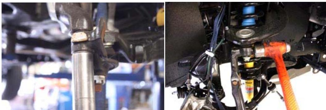
11. Guide ABS line down between the new spindle and lower ball joint/ steering stop plate. Mount new spindle, and slide lower ball joint into the double sheer mount. Attach upper ball joint to new spindle, tightening nut on ball joint, align cotter pin hole & install OEM cotter pin.
