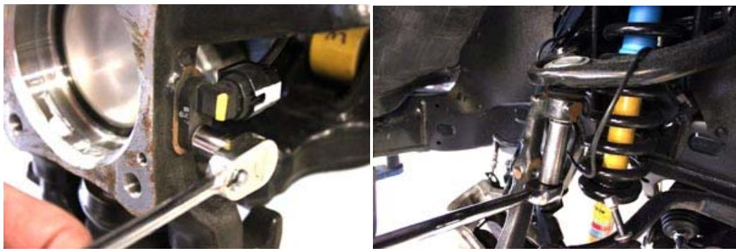
10. Remove bolts from lower ball joint / steering stop plate, then break upper ball joint loose by hitting the side of the spindle, do not hit the thread, remove stock spindle.
