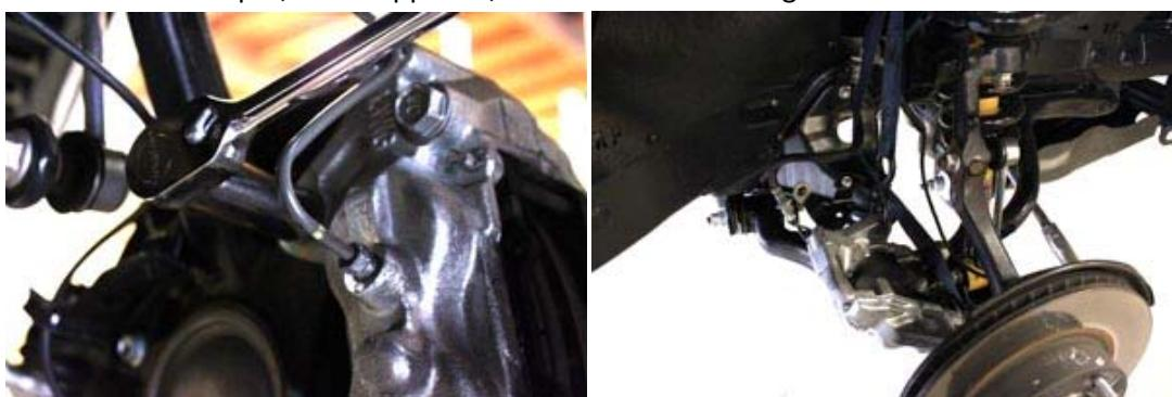
4. Remove brake rotor.
