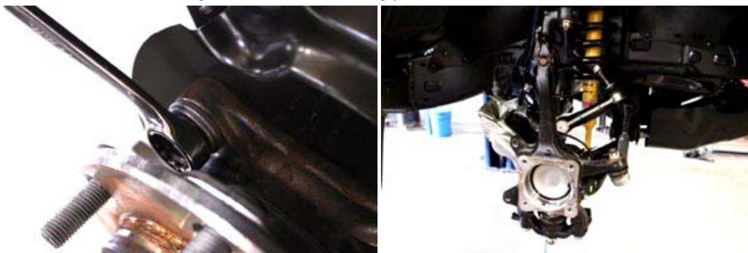
7. Remove the cotter pins from the tie rod and upper ball joint.
