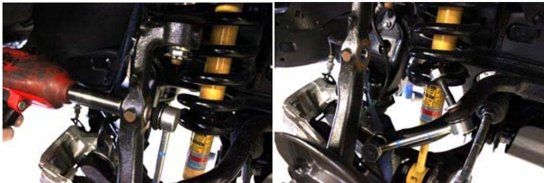
6. Remove the unit bearing, then discard backing plate & dust shield.
