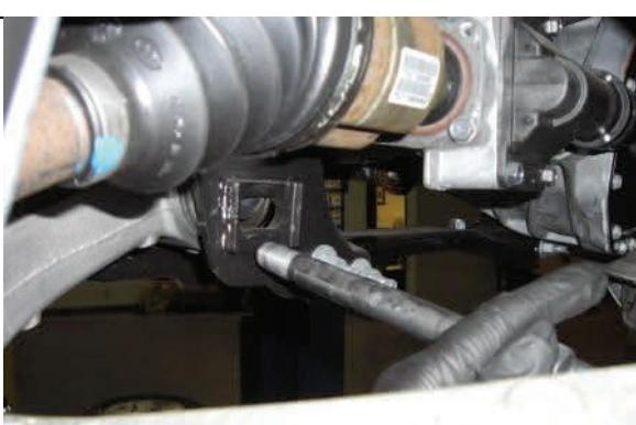
Remove lower control arm mounting bolts.
