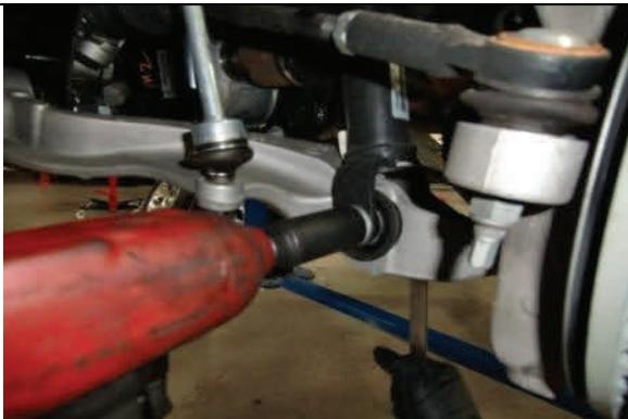
Remove lower strut mounting nut.
