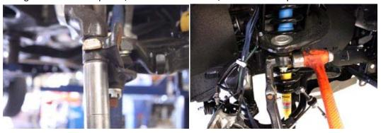
11. Guide ABS line down between the new spindle and lower ball joint/ steering stop plate. Mount new spindle, and slide lower ball joint into the double sheer mount. Attach upper ball joint to new spindle, tightening nut on ball joint, align cotter pin hole & install OEM cotter pin.
