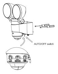
Adjustment dials are located on the backside of the motion sensor as shown in the pictures below. Rotate the motion sensor so you have access to the backside of it. This is the side that is opposite of the front, denoted by an arrow and the word FRONT on the motion sensor.
