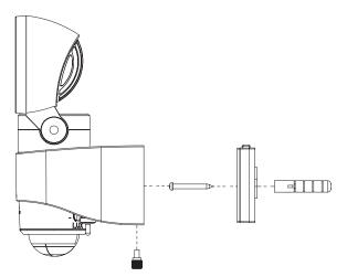
Be careful not to damage the mounting bracket as it also serves as the back of the light and the battery cover.
