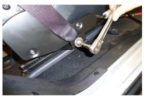
STEP 15: USING A 7/16" X 3/4" BOLT SUPPLIED IN KIT, ATTACH THE SHOULDER HARNESS TO THE OUTBOARD BRACKET.
