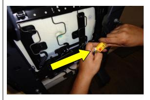
STEP 3: DISCONNECT ALL OTHER CABLES UNDER THE SEAT. (SEAT HEATER, AIR BAG, SEAT BELT SENSOR)
