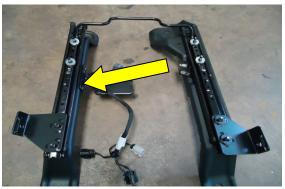
STEP 6: REMOVE FACTORY ADJUSTERS FROM FACTORY SEAT AND PLACE TO THE SIDE. DISCONNECT REMAINING SENSOR FROM THE ADJUSTERS AND RETAIN FOR LATER USE.
