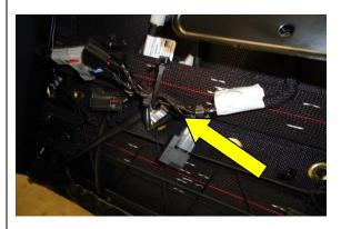
STEP 11: CONNECT THE SEAT BELT SENSOR DEVICE TO THE CABLES AND USING ZIP TIES ATTACH THE LOOSE CABLES TO THE SEAT.
