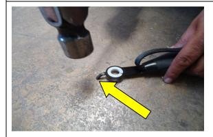
STEP 9: BEFORE ATTACHING SEAT BELT RECIEVER TO THE INBOARD SIDE OF THE SEAT, TAB MUST BE BENT FLAT.
