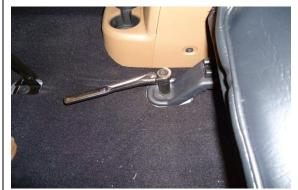
STEP 13: USING A 1/2" SOCKET WRENCH TIGHTEN FLOOR MOUNTING BOLTS.
