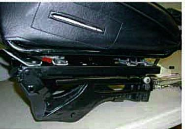
**Step # 10** Install seat belt reciever/bracket using the factory bolts. Install assembled seats and risers back into vehicle.
