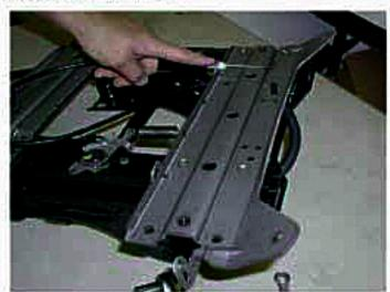
Step #7 - Install the (4) 8 mm x 1.25 x 40 studs (short threaded end, down) into the OEM riser. 4 Places.
