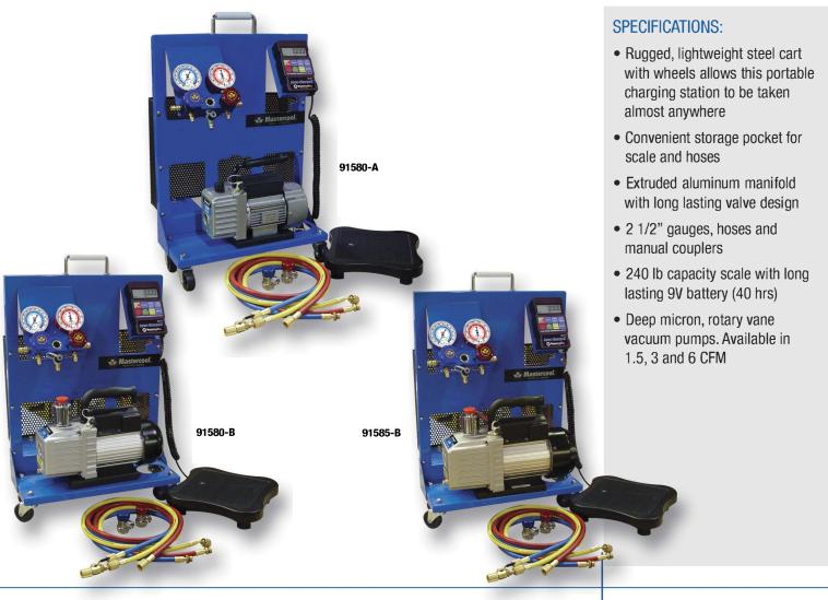
A lightweight, durable, steel frame cart that contains all the necessary tools to quickly and conveniently charge the A/C system. No need for different sized charging cylinders with Mastercool's rugged die cast electronic scale. Simply place the refrigerant cylinder on the scale and charge.
