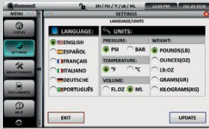
Settings Screen allows the user to select a default language, units, temperature, volume and weight measurement
