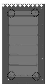
2 MARK and DRILL (4) MOUNTING HOLES [1/4-20 SCREWS]
