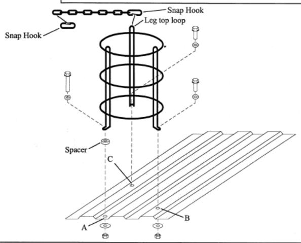
!!WARNING: SEVERE DAMAGE COULD OCCUR TO YOUR VEHICLE DURING INSTALLATION!! Look under the vehicle floor where you will be installing your freon tank ring and look for obstructions such as electrical wires, fuel lines, brake lines, fuel tank(s), spare tires, etc.
