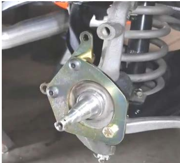
Figure 2 – Primary Caliper Mounting Bracket
