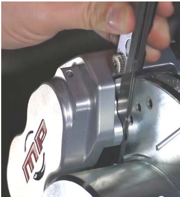
Figure 4a – Measuring the Caliper to Rotor Clearance
