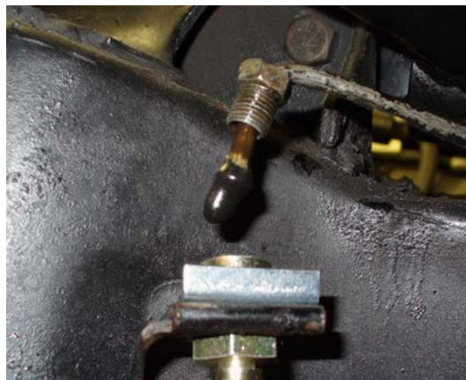
Figure 1 – Brake hose removal
