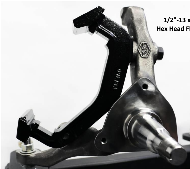
Figure 3 – Caliper Bracket Installed (Front View)
