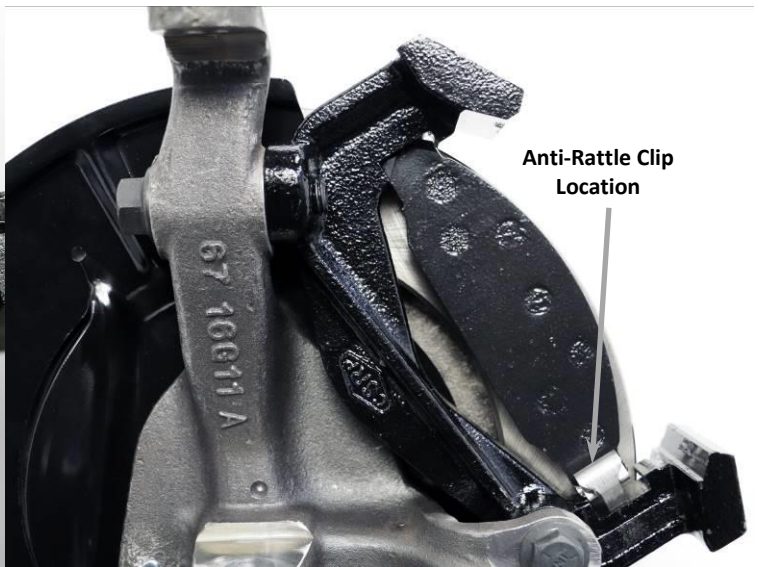
Figure 9 – Anti-Rattle Clip Location
