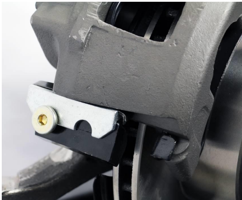
Figure 12 – Caliper Retaining Bolt Installation
