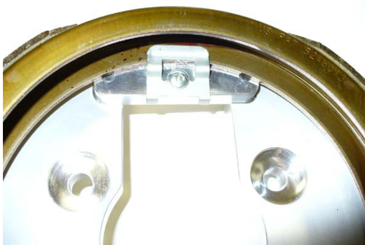
Figure 4 – Installed Park Brake Shoe Upper Retainer
