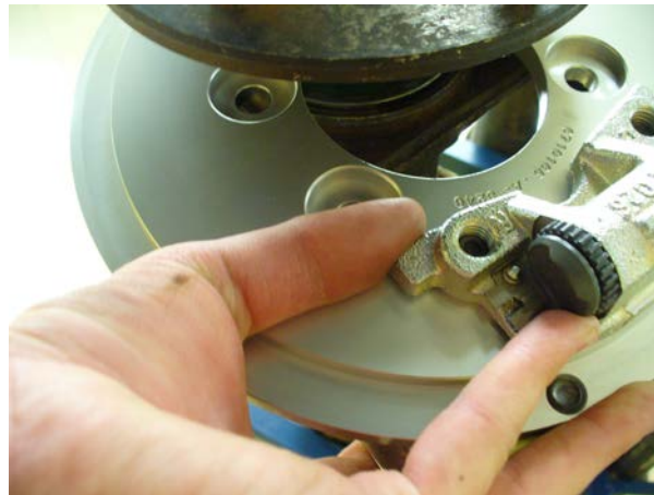
Figure 2 – Installing the Park Brake Backing Plate
