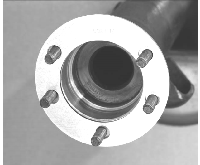
Figure 3 – Installed Spacer Flange
