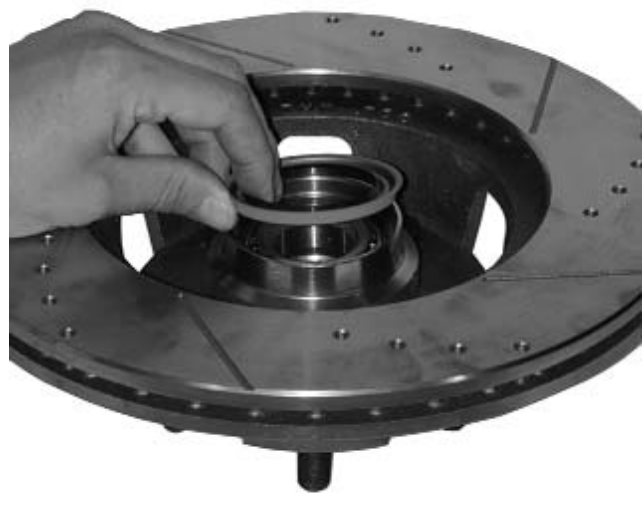
Figure 5 – Inner Wheel Seal Installation
