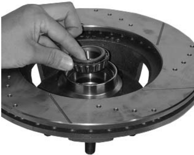
Figure 4 – Inner Wheel Bearing Installation
