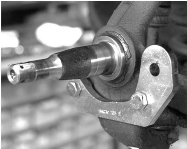
Figure 2a – Primary Caliper Mounting Bracket Installed
