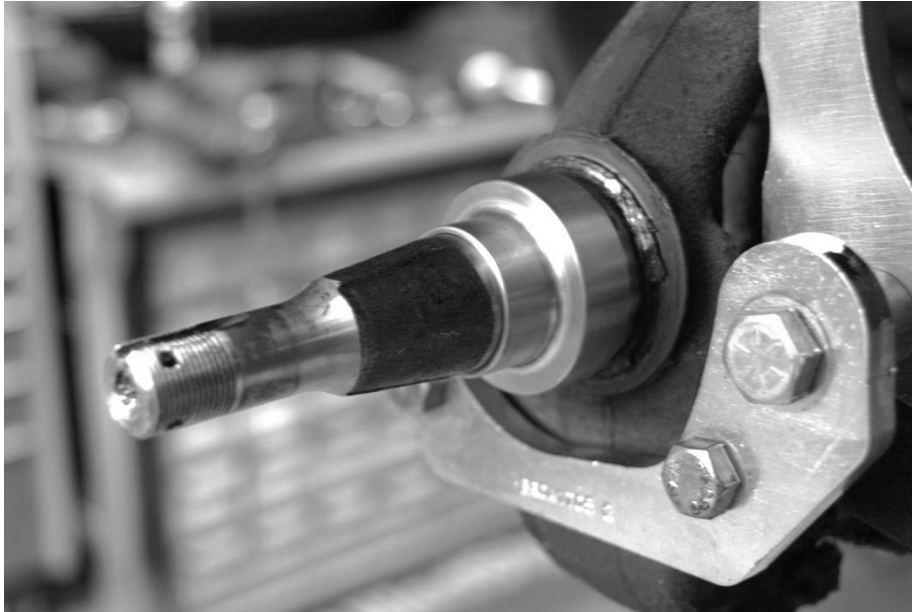
Figure 4 – Bearing Adapter Installed on the Spindle
