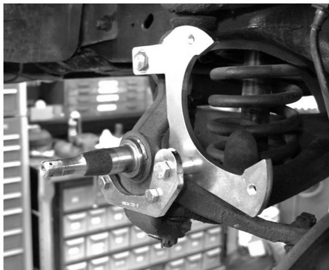
Figure 3 – Secondary Caliper Mounting Bracket Installed
