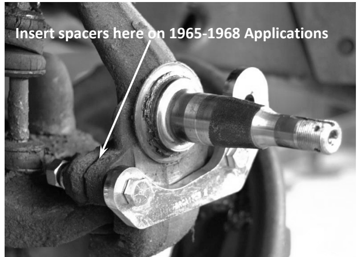
Figure 2b – Primary Caliper Mounting Bracket Installed
