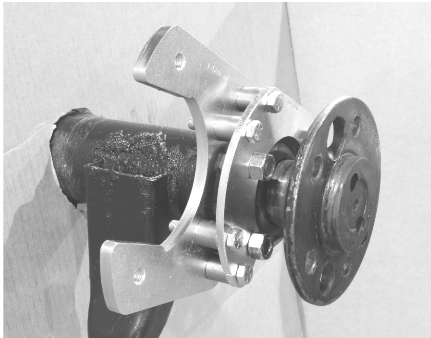
Figure 4 – Caliper Mounting Brackets Fully Installed
