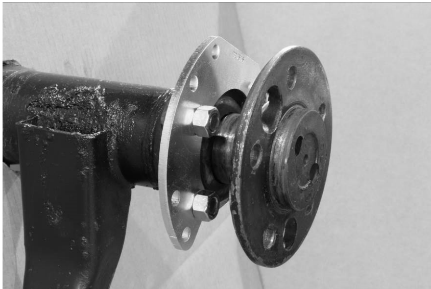
Figure 3 – Axle Re-installed w/Primary Caliper Mounting Bracket
