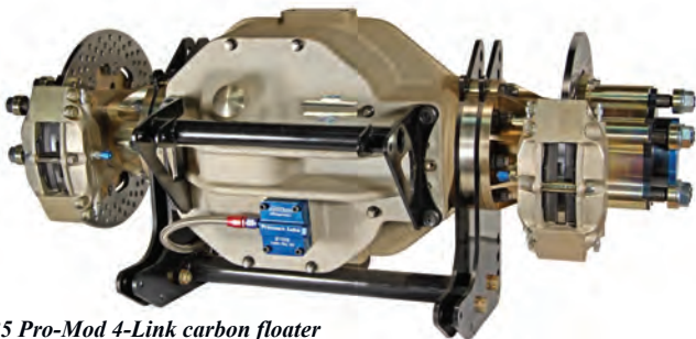
90085 Pro-Mod 4-Link carbon floater with 4130 steel brackets
