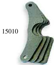
15010 Axle Mount Brackets F/C (4) 3/16 4130 welds to 1-5/8" tube axle bolts to the 35000 Torsion
