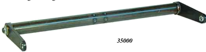
35000 Funny Car/Altered Torsion Assembly 26" centers with 5" arms
