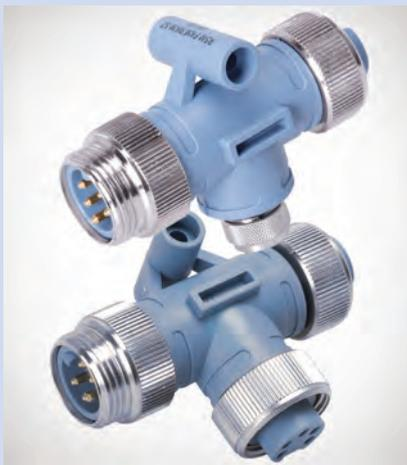
A Tee is used to tap into the trunk line for adding a drop connection. Two Mini Tees are available: 1) a Mini Tee with Mini connectors for the trunk and drop lines, and 2) a Mini/Micro Tee with Mini connectors for the trunk lines and a Micro connector for the drop line.
