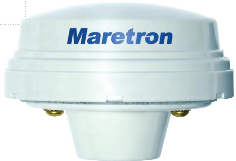
The GPS200 automatically decodes GPS correction signals from Satellite Based Augmentation Systems (SBAS) including the North American Wide Area Augmentation System (WAAS), the European Geostationary Navigation Overlay System (EGNOS), or the Asian Multifunctional Transport Satellite-based Augmentation System (MSAS) to provide better than 2.5m accuracy.
