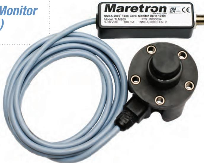
The TLM200 is mounted directly to the top of tanks using the industry standard SAE J1810 5-hole mounting pattern. The TLM200 can also be mounted to tanks with threaded tank openings using the optional 1.5" NPT adapter.
