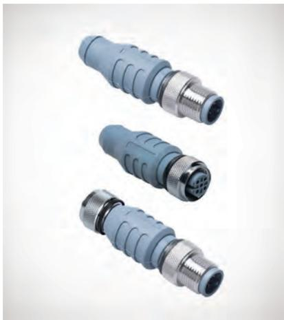
Two termination resistors are required on every NMEA 2000 network, one on each end of the trunk line. Normally, a male termination is used since male pins tend to point back to the power source. In cases where the gender is reversed, a female terminator may be required. The inline terminator is used where the network is terminated at a product, for example a GPS or weather station at the top of a mast.
