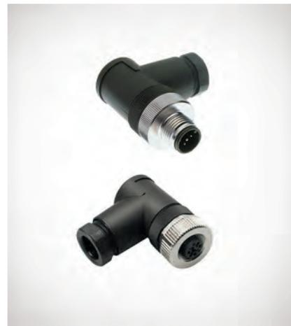
Like the straight Micro/Mid Field-attachable Connectors, the 90° field attachable connectors allow you to make field connections to bulk cable. The 90° connectors are particularly well suited for tight spaces like the back of displays where there is limited space for a straight connector.
