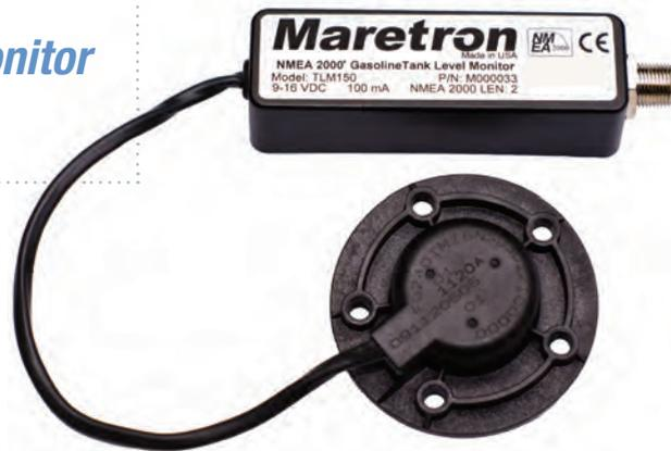
The TLM150 is mounted directly to the top of tanks using the industry standard SAE J1810 5-hole mounting pattern. The TLM150 can also be mounted to tanks with threaded tank openings using optional adapters that include both a 1.5" NPT and a 1.25" BSP adapter. The other important optional accessory for the TLM150 is the focus tube to permit use on boats with planing hulls, which is required if the vessel spends a significant amount of time with the bow pitched up.
