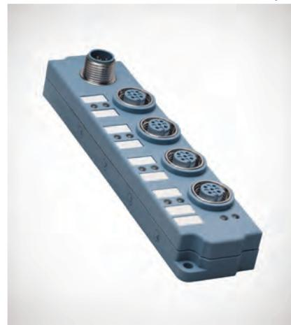
Multiport boxes allow several drop cables to be consolidated and connected back to the trunk, which eliminates the need to have numerous tees connected near a single point. Multiport boxes connect back to the trunk through a double-ended cordset and Tee.
