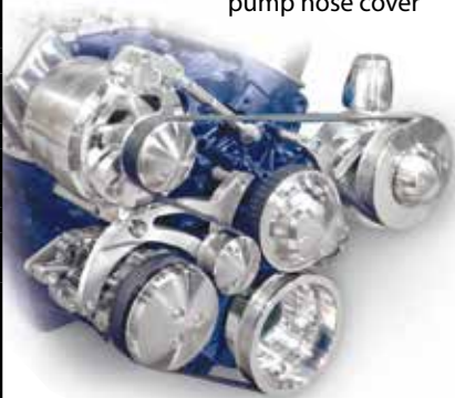
Forward Dimension 3.75" from balancer flange to water pump nose cover
