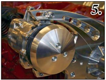
**Photo-6** Install the rear  $\frac{5}{16}$  x 2" SHCS (S155) A/C support bolt thru the rear lower ear of the A/C unit. Between the rear A/C ear and the Rear A/C support install a .200 Aluminum Bushing (AC3-.200) as shown and tighten at this time.
