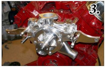
**Photo-4** Install The Main Face Plate (40721-A) using (4) (S244)  $\frac{3}{8}$  x  $\frac{3}{4}$ " SHCS thru the four counter sunk bolt holes in the front of the plate and into the four Stainless Threaded Spacers.
