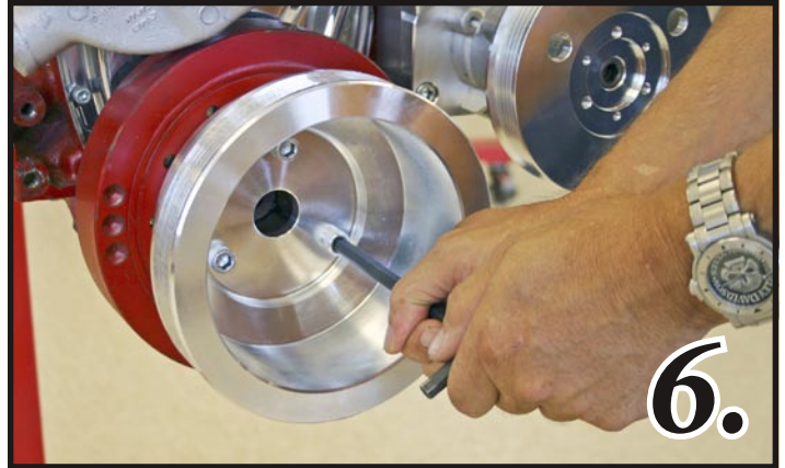
Photo 6. Apply Loc-Tite to the threads of Three \frac{3}{8} - 24 x 1" Fine Threaded Socket Cap Screws (S292) and install crank pulley (6331-A) for power steering kits or (6311-A) for Non power steering kits.
