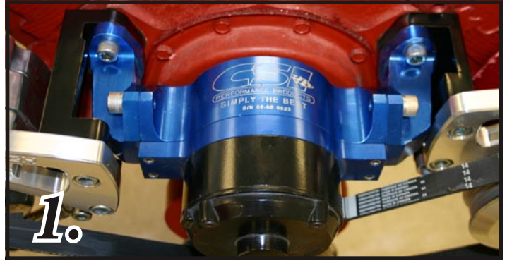
Photo 1. Ensure the sealing face of the coolant outlets are clean, flat and free of old gasket material. Using RTV Silicone Sealant and the supplied gaskets (P675) Mount Electric water pump to the block along with the Water Pump Adapter Brackets (22025-A & 22026-A) between the water pump and the block. Use (4) \frac{3}{8} - 16 x 1 \frac{1}{2} " Socket Cap Screws (S252).
