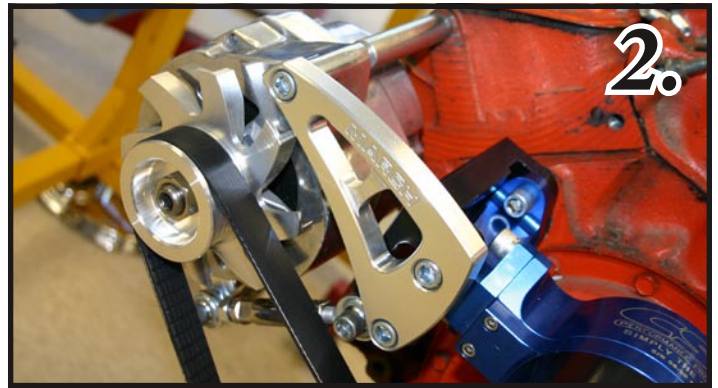
Photo 2. Mount the Front Alternator Bracket (20124-A) with (2) \frac{3}{8} - 16 x 1" Socket Caps Screws (S248). Install the alternator. Use (1) \frac{3}{8} - 16 x 6" Socket Caps Screw (S282) and (1) \frac{3}{4} " Spacer tube (TP3-3.250) between the Block and the Alternator bracket..
