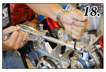
*Fig 18a.* TIP: Serpentine belt is tight when it can't be moved by more then ½ inch at it's longest span between pulleys. The belt should not be able to be twisted by more then half a turn.
