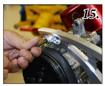
(S248)  $\frac{3}{8}$ "-16 x 1" SHCS. Place the crank pulley (7666-A) on damper and align holes. Thread the (3) screws through pulley and into damper, tighten firmly (50 ft/lbs.)
