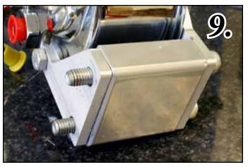
*Fig 10.* Use the (20115-C) Spacer Block between the two brackets. Install the unit to the lower right (drivers side) engine block tapped holes with (2)  $\frac{7}{16}$  x  $\frac{3^{1}}{2}$ " SHCS (S364). Then install the Power Steering pulley.
