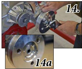
*Fig 15.* Install (S553) M8 x 1.25 x 35 mm bolt into (MM100) bushings as shown. Install one each into Alternator, and A/C units in adjustment slots, leave loose at this time.
