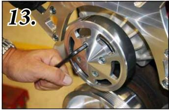
Fig 14. Install power steering pulley. (618-A or 535-A) Mount pulley in-line with crank pulley. Press on with a %16" wrench and install tool. When properly installed, pulley should be flush with top of shaft as shown. Fig 14a.
