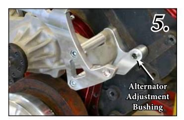
*Fig 6.* Install the Alternator (P572) using a  $\frac{3}{8}$ x  $4\frac{3}{4}$ " SHCS (S277) and the billet spacer bushing (A3-1.250). Adjust Bushing (S452) to take up any space between the lower alternator support and the spacer. (snug only at this time). Tighten lightly at this time.
