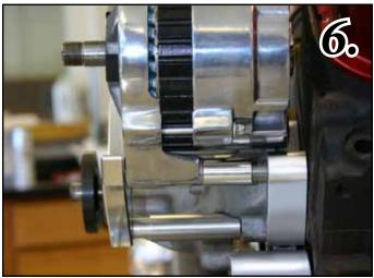
*Fig 7.* Install A/C unit (P412) Using a M8 x 20mm SHCS (S550) in the lower front hole and a  $^5/_{16}$  x  $1^1/_{2}$ " (S150) SHCS in the rear lower Hole. Use a  $^3/_{8}$ " I.D. x .300 long spacer (TP3-.300) between the rear A/C bracket and the rear ear of the A/C unit As Shown.
