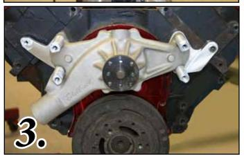
*Fig 4.* Install Main Front Bracket (21201-A Style Track) or (21261-A Revolver) to the threaded studs using (4) 3/8 -16 x 1" socket caps. (S248)
