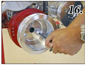
*Fig 17.* Install alternator fan (221-A) and pulley (206-A) Along with Lock Washer (S685) and tighten pulley nut (impact to 90 ft, pounds). Install Alt Cap (306-A) with (3) 8-32 x 1" SHCS (S028). Place the compressor clutch cover (394-A) onto the compressor clutch and align. Thread the three (3) (S520) M6 - 1.0 x 16mm Button Head Bolts. through the cover and into the clutch and tighten. Caution – Do not over-tighten!
