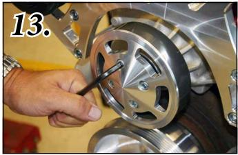
*Fig 14.* Install power steering pulley. (618-A or 535-A) Mount pulley in-line with crank pulley. Press on with a %6'' wrench and install tool. When properly installed, pulley should be flush with top of shaft as shown. *Fig 14a.*
