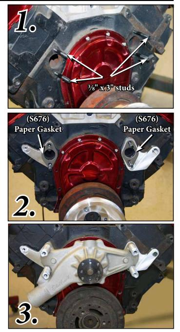
*Fig 4.* Install Main Front Bracket (21201-A Style Track), (21261-A Revolver) or (21216-A Pro-Track) to the threaded studs using (4)  $\frac{3}{8}$  -16 x 1" socket caps. (S248)
