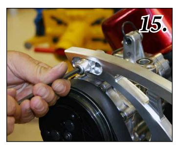
(S248) <sup>3</sup>/<sub>8</sub>"-16 x 1" SHCS. Place the crank pulley (7666-A) on damper and align holes. Thread the (3) screws through pulley and into damper, tighten firmly (50 ft/lbs.)
