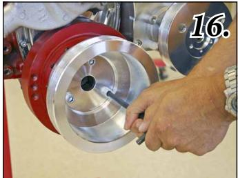
*Fig 17.* Install alternator fan (221-A) and pulley (206-A) Along with Lock Washer (S685) and tighten pulley nut (impact to 90 ft, pounds). Install Alt Cap (306-A) with (3) 8-32 x 1" SHCS (S028). Place the compressor clutch cover (394-A) onto the compressor clutch and align. Thread the three (3) (S520) M6 - 1.0 x 16mm Button Head Bolts. through the cover and into the clutch and tighten. **Caution – Do not over-tighten!**
