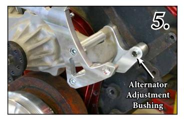
*Fig 6.* Install the Alternator (P572) using a  $\frac{3}{8} \times 4^{\frac{3}{4}}$ " SHCS (S277) and the billet spacer bushing (A3-1.250). Adjust Bushing (S452) to take up any space between the lower alternator support and the spacer. (snug only at this time). Tighten lightly at this time.
