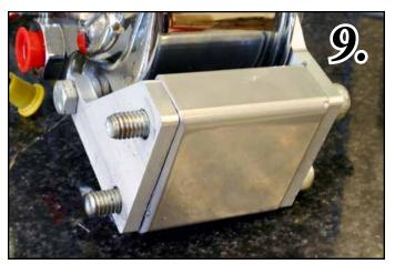
*Fig 10.* Use the (20115-C) Spacer Block between the two brackets. Install the unit to the lower right (drivers side) engine block tapped holes with (2)  $\frac{7}{16} \times \frac{3^{1}}{2}$ " SHCS (S364). Then install the Power Steering pulley.
