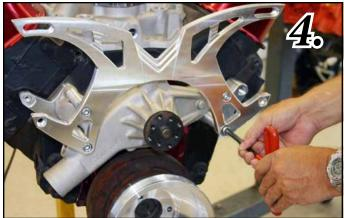
*Fig 5.* Install <sup>5</sup>/<sub>8</sub>"-18 Threaded Alternator Adjustment Bushing (S452) into Rear Alternator Support Bracket as shown.
